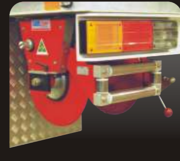
Underslung Hose Reel mounted on a fire truck
